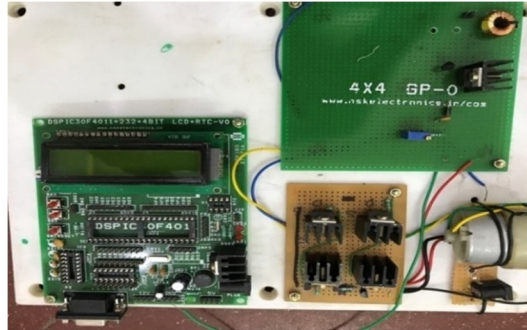
Figure 2. Hardware Implementation of ACU for Door Latch control
